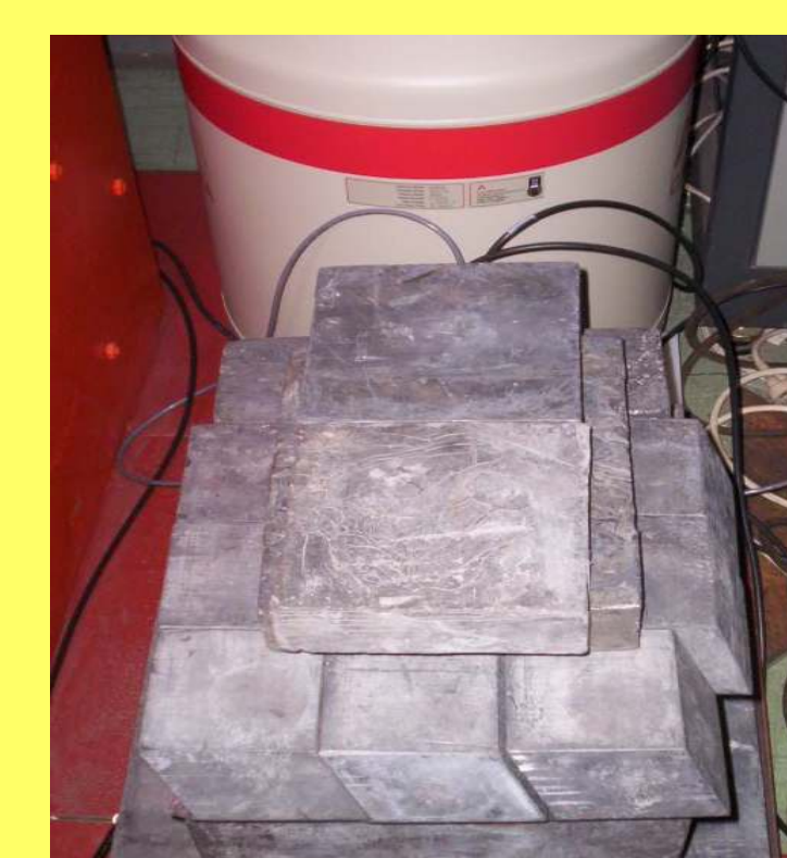
Figure 4. The HPGe detector situated inside the simple shield.
