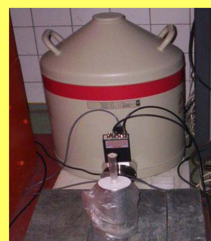
Figure 2. The HPGe detector situated outside the simple shield.
